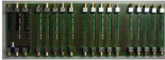
▲ Fig. 4 Test PCB containing various via geometries.
