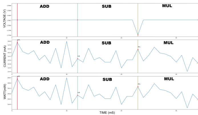
Fig. 4. 1.8 V ADC Measurements for ADD, SUB and MUL
