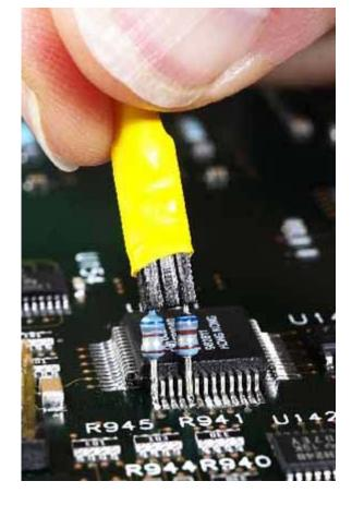
The coaxial resistor is able to make contact with an individual package lead without bridging over to adjacent pins. The illustration shows a closer view of the electrical connection.
