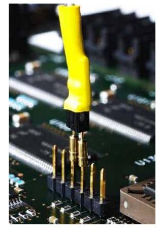
Electrically, this connection (including the original 0.025-in. pins) presents only a 1.1-pF equivalent capacitive load on the target.
