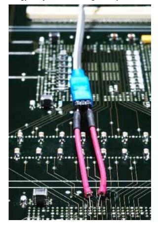
The figure above shows a damped wire accessory soldered to the breakout vias of a 1-mm-pitch BGA. The accessory (red) simply slides into the receiving socket of the probe tip (blue).
