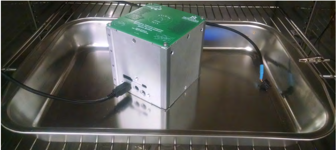
Figure 4.15: Fully Assembled Artemis ready for Thermal Test
