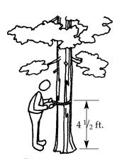
DBH is measured  $4^{1}/_{2}$  feet above the ground.
