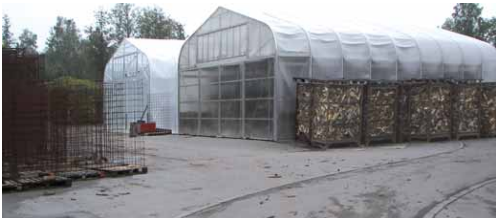
Figure 4.9.3 Greenhouses for drying log woods at the Biomassehof Allgäu (Bayern - DE)
