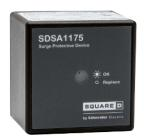
Surge protection device, Surgelogic, 36kA, 120/240 VAC, 1 phase, 3 wire, 25kA SCCR, NEMA 4X
