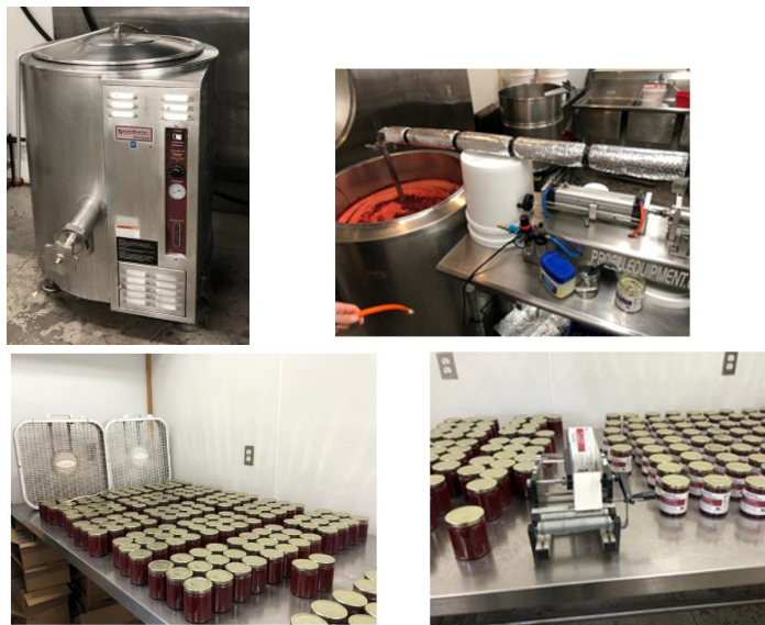
Fig. 1. Preserves manufacture steps include cooking (40 Gallon SteamMaster kettle), filling, cooling, and labeling.
