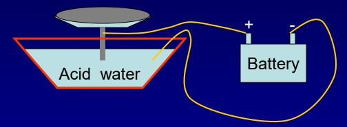
Carbon granules (variable resistor)
