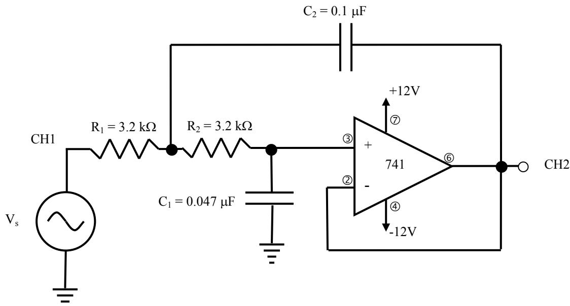
Use the function generator and the oscilloscope to observe simultaneously the source voltage (CH1) and the voltage at the op amp's output (CH2), and fill out the table on the next page.
