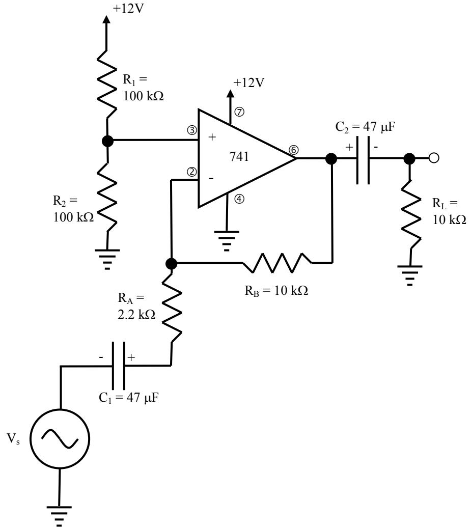
Describe your observations of how this circuit behaves. What does the output waveform across  $R_L$  look like compared to the input waveform from  $V_s$ ?
