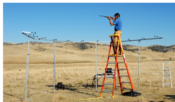
Figure 2: Recording apparatus with semicircular arc of twelve microphones elevated 3 meters, and marksman positioning firearm muzzle at center of arc.
