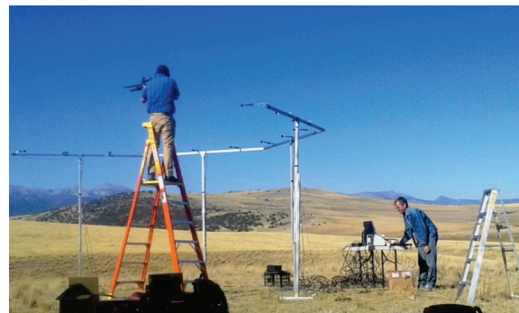
Figure 2: Test configuration with microphones and firearm elevated for quasi-anechoic recording.
