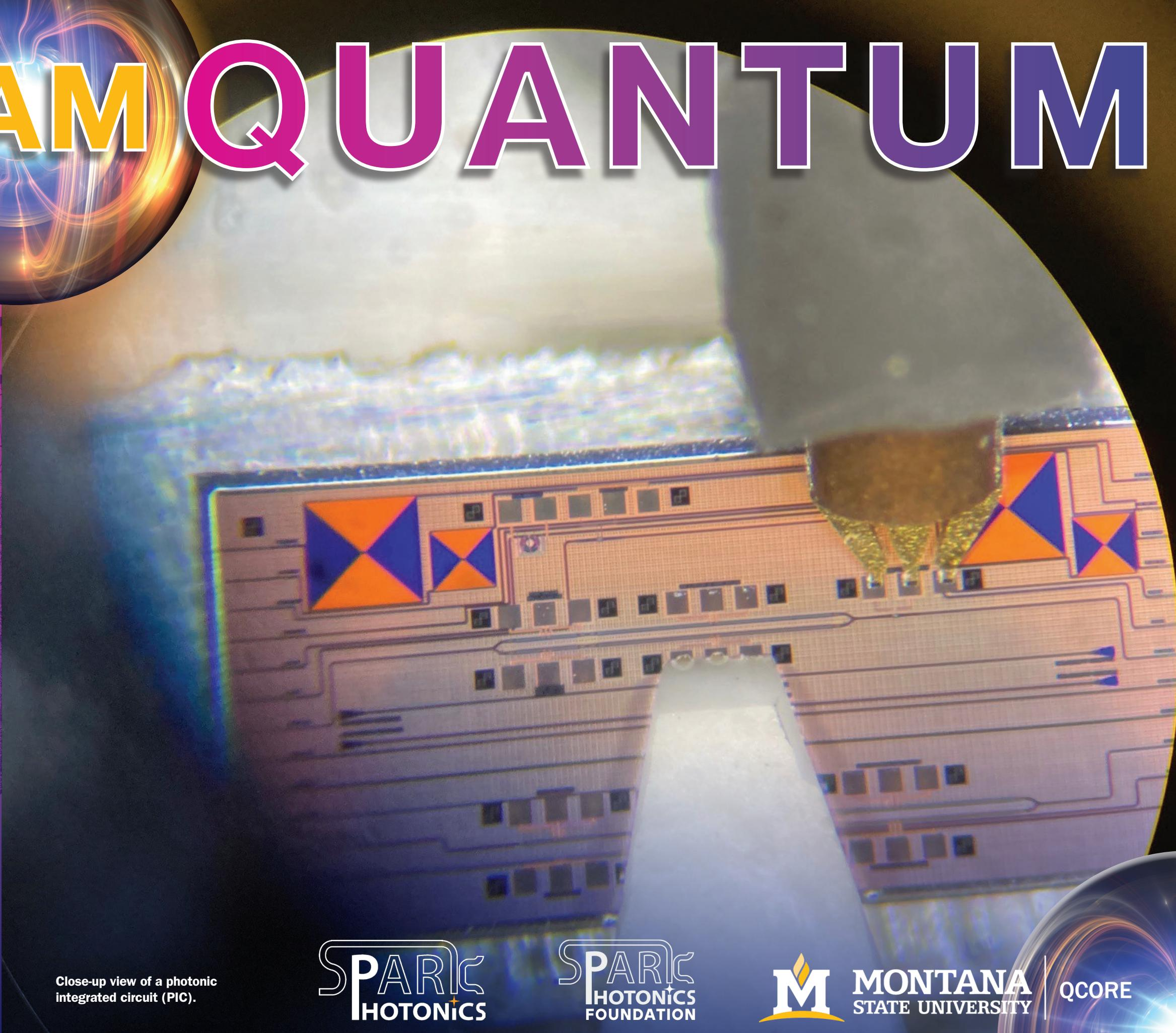
Close-up view of a photonic integrated circuit (PIC).
